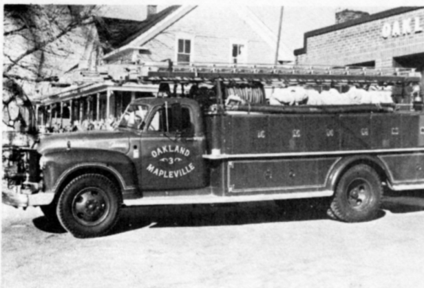
Engine 3: 1952 Chevrolet, 800 gallon tank, 500 gpm pump, bought from Glendale Fire Department in 1975.
