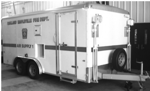
Air Supply Trailer Purchased With A National Fire Grant For $75,000, Has Air Compressor And Cascade System To Fill SCBA Bottles And A 12KW Generator.
